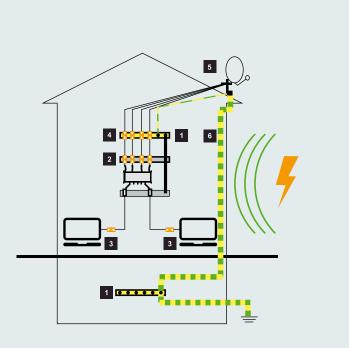
Should a risk analysis according to VDE 0185-305-2 (IEC/EN 62305-2) not be possible or not be required by the authorities, then static atmospheric surge voltages (e.g. lightning) can cause arcing from the 16 mm<sup>2</sup> earthing conductor to the electrical installation or the antenna system of the building. For this reason, we recommend making the earthing conductor insulating and resistant to high voltages and floating discharges through suitable measures.
