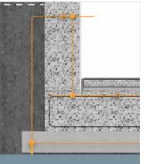
White trough, pressurised water-tight ring earth entry in the groundwater
