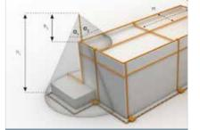
The protective angle method is suitable for buildings with simple shapes.
