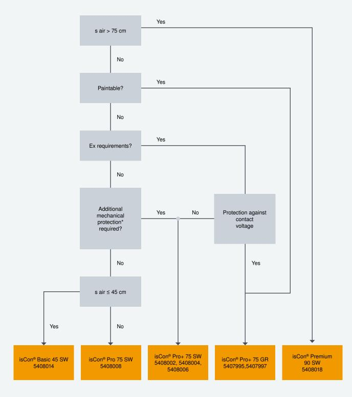
\*Additional mechanical protection: Surface damage of the external protective jacket does not influence the high-voltage-resistant, insulating function of the black isCon® Pro+ down-conductor! For this, the jacketing must remain for a minimum of 0.2 mm over the entire scope of the down-conductor.
