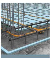
Insulated floor plate with perimeter insulation (here: shown in blue)
