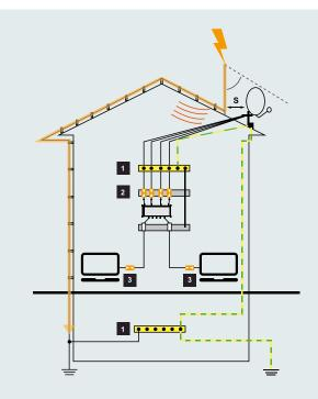
Current path in case of a direct strike close to a satellite dish
