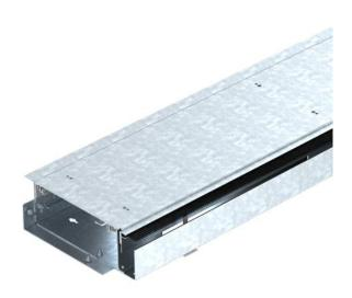
Ready-to-mount trunking unit for cable routing and device installation, consisting of a trunking base with two covers and a height-adjustable brush bar. The scope of delivery contains two lid butt seals and one connector. For height adjustment, six height adjustment units are required. Load capacity up to a maximum of 5 kN. The trunking unit can be supplemented with an adjustable covering contact profile for screed limitation in areas of door soffits and in front of radiator alcoves.
